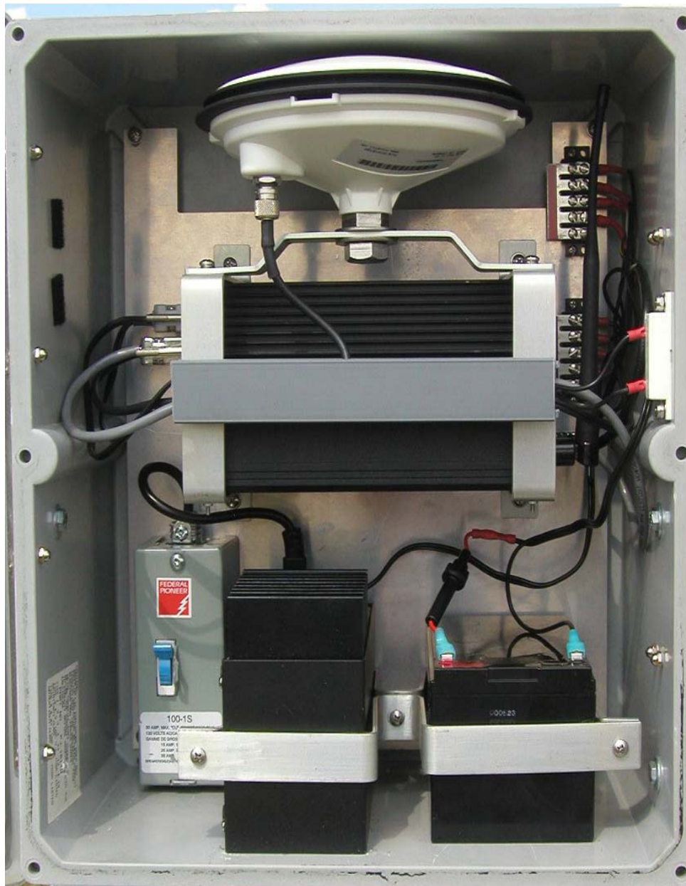
Figure 3.6: GPS Hardware Package (cover removed)
